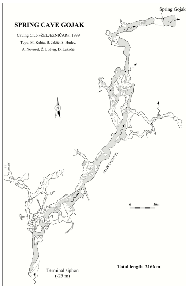
Fig. 3 Topographic plan of the Spring Cave Gojak
